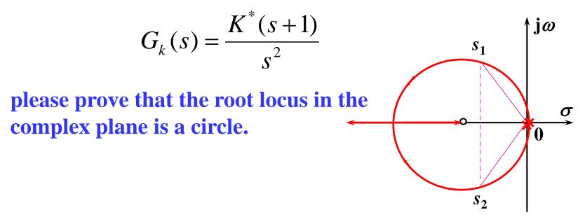
**Conclusion:** For the open-loop transfer function with one zero and two poles, the root locus of characteristic equation is probably a circle in the complex plane.
