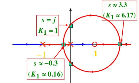
For  $K_g$  varying from  $-\infty \rightarrow 0$  together with  $K_g = [0, +\infty)$  simultaneously, the root loci are named the "complete root loci".
