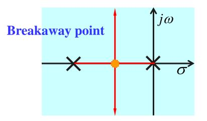
When the root locus has segments on the real axis between two poles, there must be a point at which the two segments break away from the real axis and enter the complex region.
