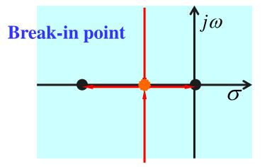
For two finite zeros or one finite zero and one at infinity, the segments are coming from complex region and enter the real axis.
