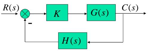
We have seen how this form of feedback is able to minimize the effect of disturbances.
