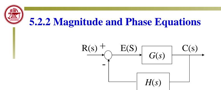
**Characteristic equation of closed-loop transfer function**
